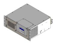
DryLine® Dehydrator, Low-pressure membrane, 19 in rack mountable, Wall mountable, Cut-in at 2.0 psi, Cut-out at 5.0 psi, with discrete and summary alarms, 115/230 Vac, 50/60 Hz
