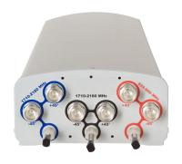
6-port sector antenna,  $2x\ 824-960$  and  $4x\ 1710-2180$  MHz,  $65^\circ$  HPBW, RET compatible
